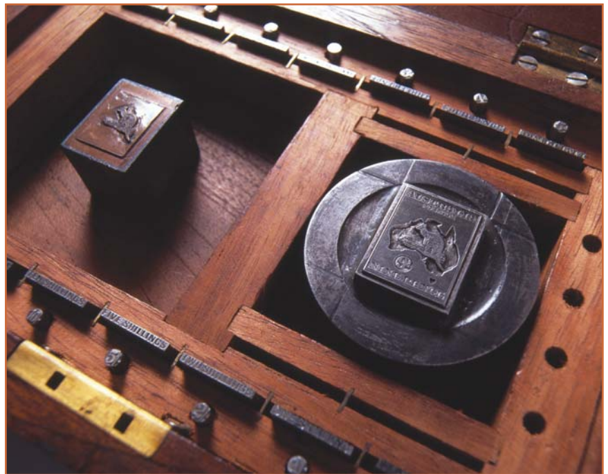
The master die of the Kangaroo and Map stamps includes interchangeable plugs for the denominations and an electro of the vignette for printing the second colour of the high-value stamps
